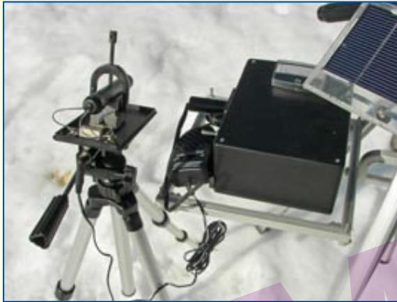
One laser experiment was a solar supercapacitor setup for distance ignition of black powder. Black powder has an ignition temperature of around 630°F, depending on the exact composition of the powder. We tested the ignition capability of a 200 milliwatt red
