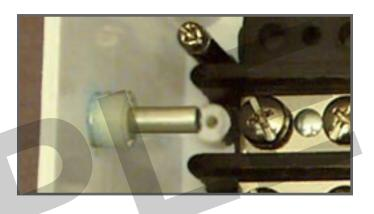
Process control box pressure sensor port (above), and with pressure sensor installed (below)
